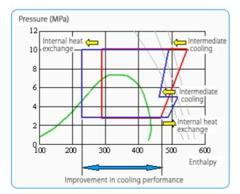
When the transcritical  $CO_2$  refrigeration cycle is applied in refrigerator and freezer equipment, the theoretical efficiency (COP) is said to be generally lower than that of HFC. An effective way to offset this is to employ: 1) an internal heat exchanger, and 2) an intermediate cooler.
